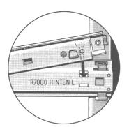
Push the front of the telescopic guide lug down onto the square hole in the front of the support rail.
